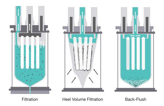
The unique FUNDALOOP® design allows for performing single-cycle and multi-cycle filtrations, where the cake can be back-flushed and accumulated on the bottom of the bag. Finally the compressed bag containing the solid waste is removed and safely disposed of in a very compacted form.
