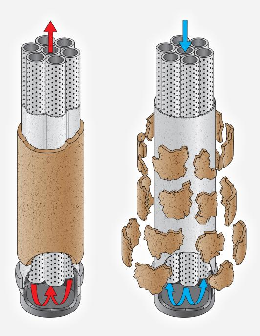
Formation and drying of the filter cake with the automated STERIBAC® candle filter system.
