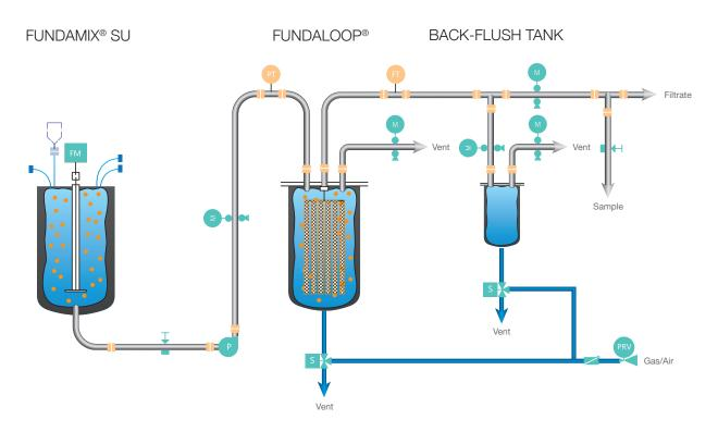
Typical process flow diagram of a FUNDALOOP® filter for high capacity filtration and a FUNDAMIX® SU mixer.
