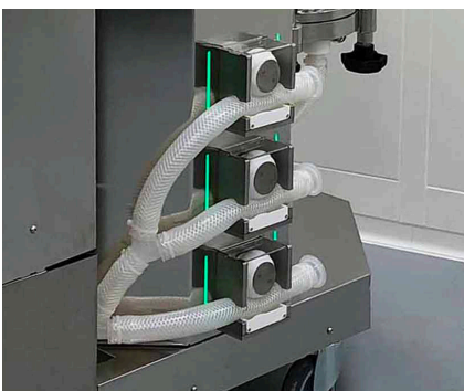
FUNDALOOP® 3000 single-use filter skid employing multiple SU valves for full flow control.
